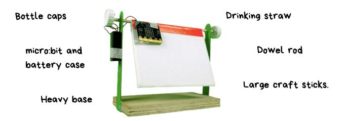
Attach the micro:bit to the flap as shown in the picture and tape the battery case to the side. Put your anemometer outside with the Wind behind the moving flap. Press button A to start collecting Wind force data. Press button B to stop or pause.
