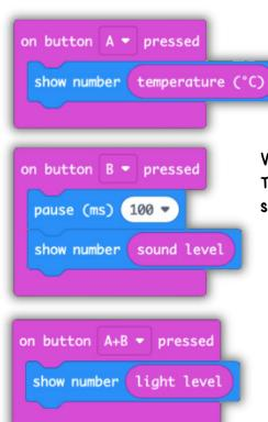
When you press button A, the temperature will show on the LED display.
