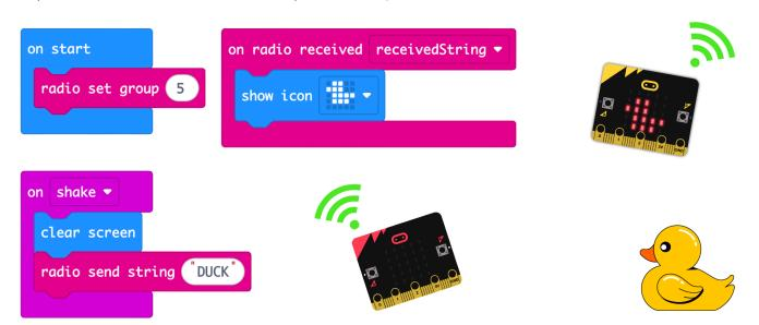
Now flash the code to both micro:bits and attach the battery power packs. Give one micro:bit to your friend and take it in turns to teleport the duck by shaking your micro:bits!
